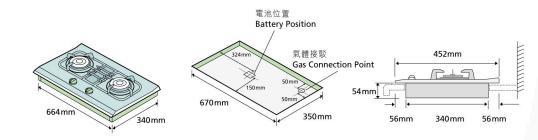
^ RRDB62S亦可安裝於703 x 403毫米的櫃面開孔 RRDB62S can also be installed in 703 x 403mm bench top cut-out
