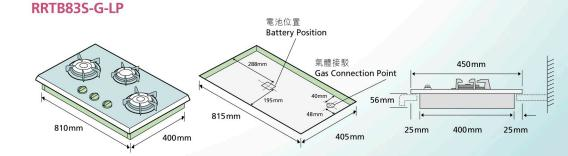
\* 平面爐與牆身須保留最少100毫米距離 Recommend to reserve a minimum 100mm distance (depth) between hob and wall
