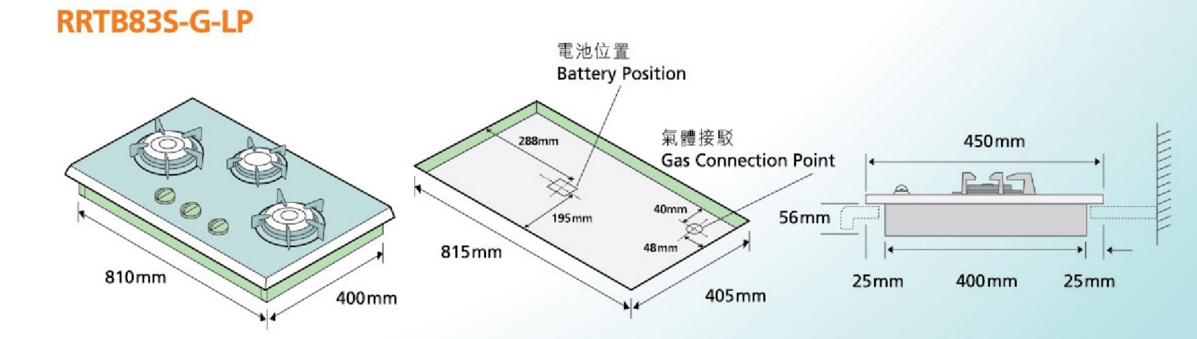
\* 平面爐與牆身須保留最少100毫米距離 Recommend to reserve a minimum 100mm distance (depth) between hob and wall
