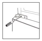
10.Unscrew right middle stopper with metal block from bottom of upper door. And then install left middle stopper and metal block in left side of bottom of upper door.
