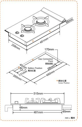
\* 高度至爐架 (至廚櫃面) Height to pan support (to bench top)
